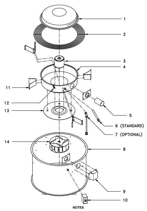
Fan shown is standard unit. Units built for restaurant service do not have internal wiring post (No. 7) or birdscreen (No. 2). Unit shown is RG model with UL762 and externally mounted disconnect switch. RF units (UL705) have disconnect switch mounted internally.
