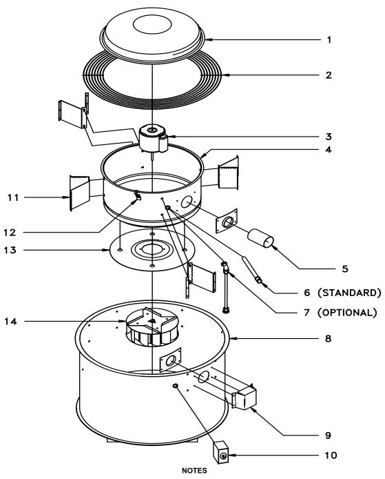
Fan shown is standard unit. Units built for restaurant service do not have internal wiring post (No. 7) or birdscreen (No. 2). Unit shown is RG model with UL 762 and externally mounted disconnect switch. RF units (UL705) have disconnect switch mounted internally.
