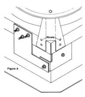
Attach the hinge bracket to the fan curb and orifice section by drilling three holes per side using the bracket as a template as shown in Figure A. Use three 5/16 x 3/4 inch bolts, and locknuts. Place the bolt head to the inside. The edge of the bracket should just cover the rivets.
