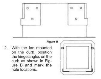
3. Drill 3/8 inch holes at the locations marked on the curb. Attach the hinge angles to the curb using 5/16 x 3/4 inch bolts and locknuts. Place the bolt head to the outside.
