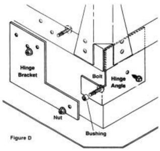
6. Place the fan complete with hinge bracket and eyebolt on the curb so that the hinge brackets and hinge angles align properly. Using the 5/16 x 1 inch bolts, bushings, and nuts as shown in Figure D, connect the hinge brackets to the hinge angles.
